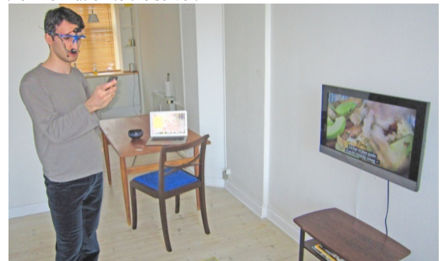
Figure 2. An example of a potential multi screen scenario with a user wearing a HMET, and able to interact with a TV screen (on the wall), a computer screen (on the table) and a mobile phone.
