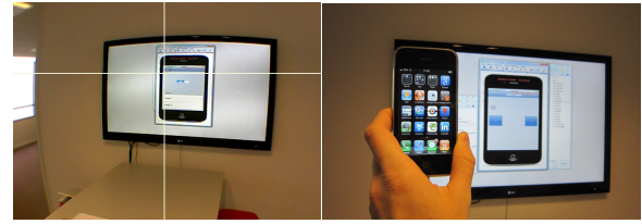
Figure 10 Interaction with iPhone emulator. Left image shows the scene image with the gaze point (white cross), and the right image shows the visual appearance of a real iPhone and the emulator in the user's field of view are about the same.
