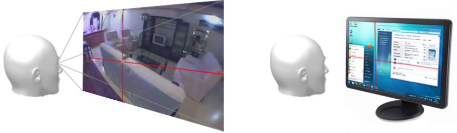
Figure 1.7: (left) RGT estimates the gaze point in a fixed two-dimensional space e.g., computer display. (right) In contrast, HMGT estimates the gaze in the user's FoV.
