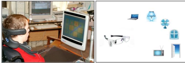
Figure 1.2: (left) Gaze-based interaction with one computer display using RGT (right) mobile gaze-based interaction with objects in the environment using HMGT.
