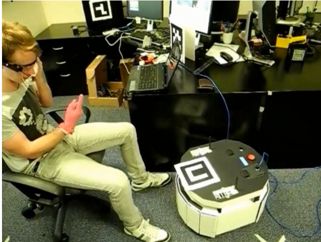
Figure 8. System At Work. This figure shows the user gazing at the visual marker, identifying the robot. A hand gesture is performed to transmit a movement command to the robot.
